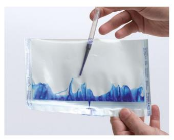
2. Faulty sealing seam: The test ink penetrates the sealing seam (e.g. channel). The sealing device should be checked (if necessary) and the test schould be repeated.
