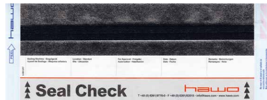
1. Intact seal for a specified seal width in accordance with EN ISO 11607-2
