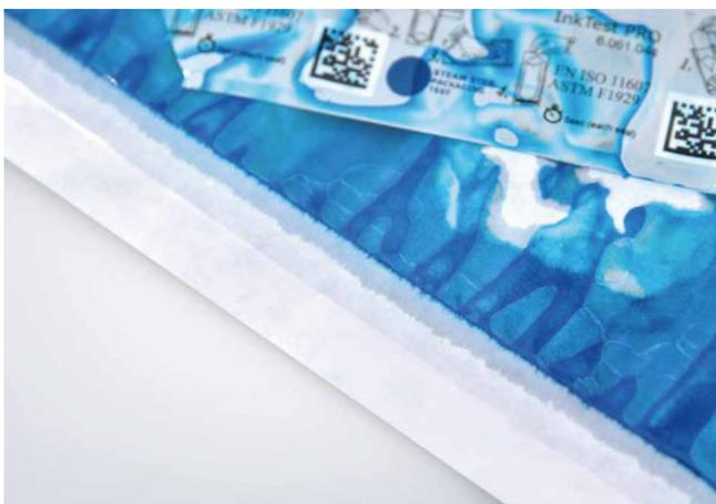
**1. Intact sealing seam:** The test ink does not penetrate the sealing seam. Hence, the sealing seam complies with the specification.
