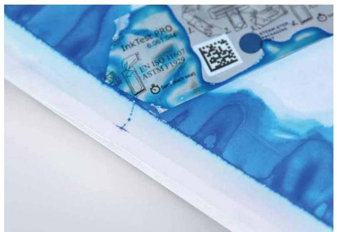
**2. Faulty sealing seam:** The test ink penetrates the sealing seam (e.g. channel). The sealing device should be checked (if necessary) and the test should be repeated.
